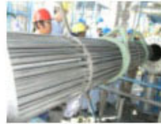
Re-refining 500 kW, 650 °C Preheating of fuel oil Flange : DN350
