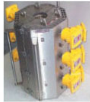
Industrial oven, 3 zones ATEX, 1.5 kW Hydrocarbons cracking
